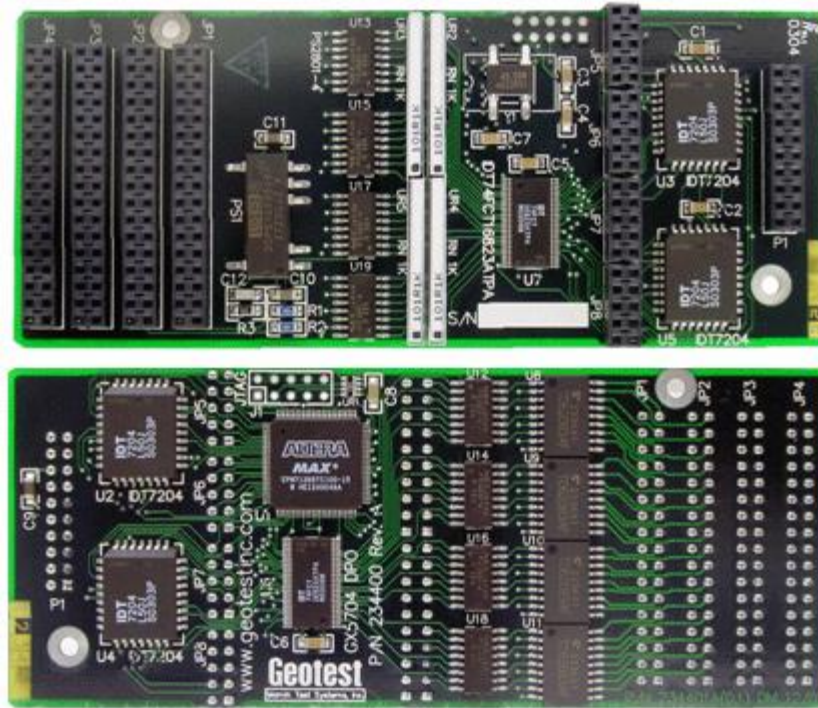
Figure 2-10: GX5704- Digital Power Output (DPO) Module
